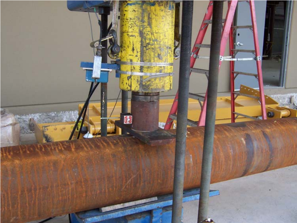
Figure 1 - Dent installation rig to install dents
