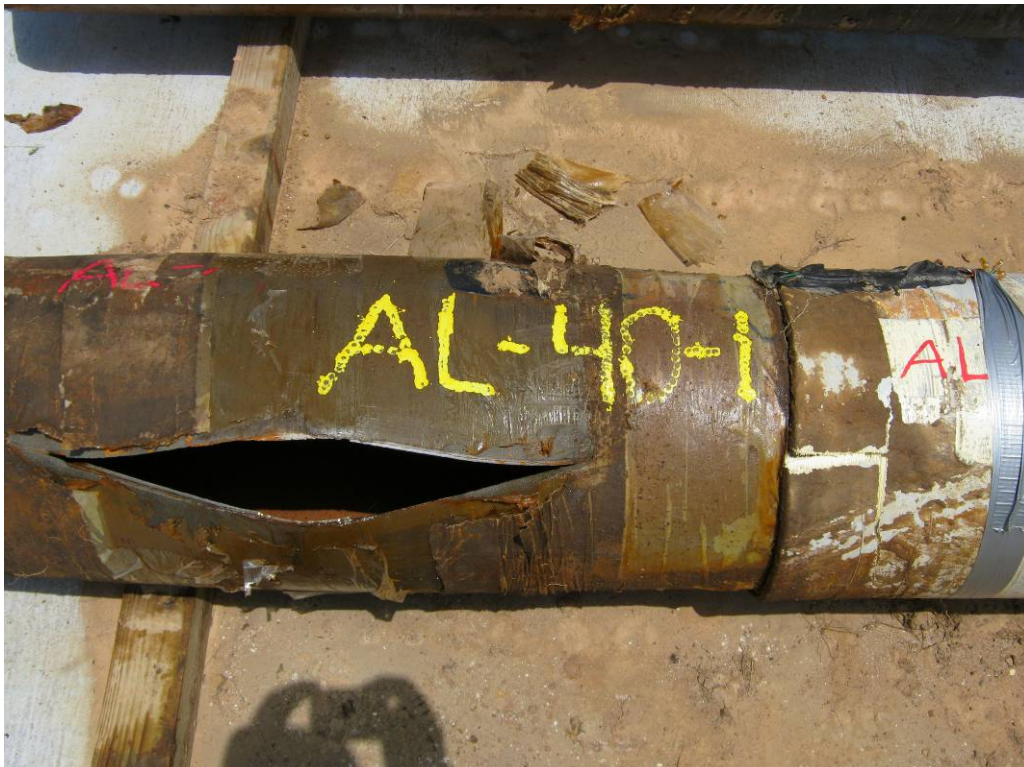
Figure 4 – Photograph of Failure Location, 40% Corrosion Sample
