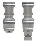
The Hollow or Solid Plug provides the pressure seal in the access fitting and is the carrier for the corrosion monitoring device (probe or coupon holder). The primary packing and guide rings are made from PTFE (15% glass filled) as standard but are available in a range of materials including metal seals for high temperature service.
