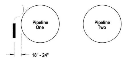
**Example 2**: Single Reference Electrode, Two Parallel or Crossing Pipelines
