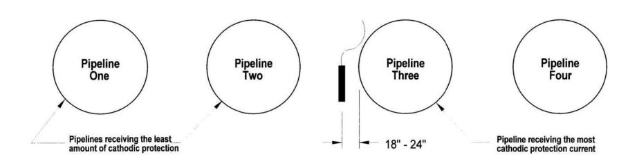
Example 4: Single Reference Electrode, Multiple parallel pipelines.
