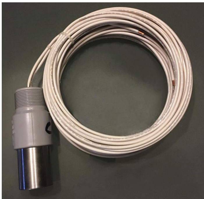
Exterior corrosion coupon for monitoring cathodic protection of platforms (100 cm 2 ) with 10 AWG THHN-THWN wire.
