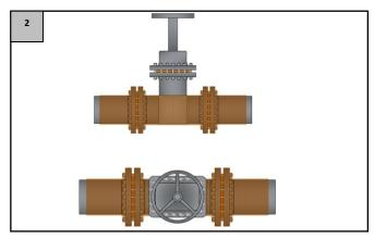
Apply a homogeneous layer of 2 to 8 mils of tecnolato-primer over all of the surface to cover.
