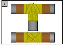
Tighten the tape while placing it in the shape of a cross, as shown in the picture.
