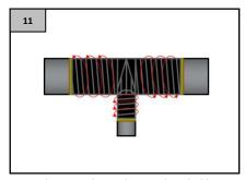
Cover the pipe, placing the tecnolato-shield strips with a 50% overlap, making sure that no air bubbles are generated. If it is necessary, make cuts on the tape to avoid that part of it lifts.
