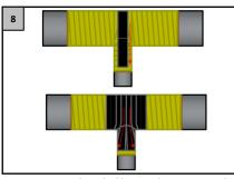
Cut some tecnolato-shield trips, beginning at the center with a 50% overlap, making sure that no air bubbles are generated. If it is necessary, make cuts on the tape to avoid that part of it lifts.
