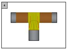
Beginning at the center, apply the strips with a 50% overlap, making sure that no air bubbles are generated. If it is necessary, make cuts on the tape to avoid that part of it lifts.
