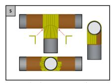
To ensure that there are no uncovered areas, cut some strips of tecnolato-tape and apply them on the angle between pipes, as shown in the picture above.
