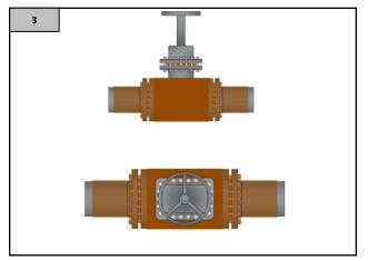
$\mbox{{\it Fill}}$  in the área betweem the internal faces of the flanges with tecnolatomastic forming a circle.
