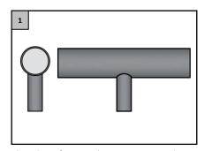
Clean the surface according to SSPC SP1 – solvent cleaning. Prepare the surface with hand or power tool cleaning, removing all the calamine, oxide, paint and other contaminants according to SSPC SP2/SP3.
