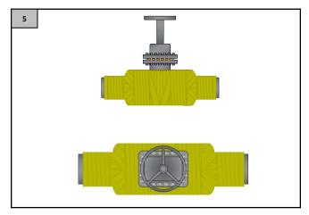
Put the tecnolato-tape starting in the center of the valve and then cover the sides crisscrossing the tapes until there are no areas left to cover.
