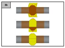
As an alternative to step 3.a., cut a tecnolato-tape strip that is long and wide enough to cover the entire flange, as shown in the picture.
