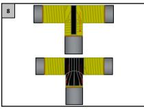
Cut some tecnolato-shield trips, beginning at the center with a 50% overlap, making sure that no air bubbles are generated. If it is necessary, make cuts on the tape to avoid that part of it lifts.
