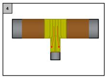
Beginning at the center, apply the strips with a 50% overlap, making sure that no air bubbles are generated. If it is necessary, make cuts on the tape to avoid that part of it lifts.
