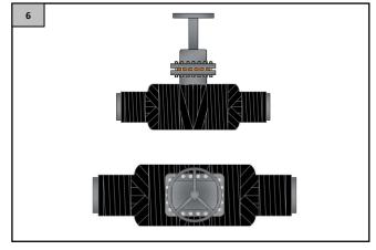
Place the tecnolato-shield starting in the center of the valve and then cover the side crisscrossing the tapes until there are no areas left to cover. Cut strips of tecnolato-shield. starting from the center place tapes adjacents with an overlap of 50% ensuring that there are no areas with air pockets, if necessary make cuts in the tape to avoid lifting.
