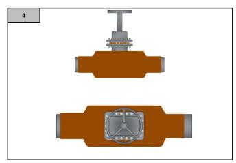
Apply the tecnolato-mastic forming an angle of approximately  $45^{\circ}$  between the flange border and the pipe.
