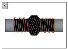
Cover the pipe with tecnolato-shield strips, beginning at the center, placing them with a 50% overlap, and making sure that no air bubbles are generated. If it is necessary, make cuts on the tape to avoid that part of it lifts.
