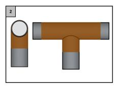
Apply a homogeneous layer of 2-8 mil of tecnolato-primer over the surface to be covered.
