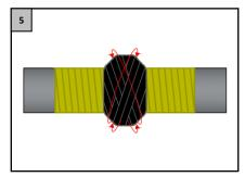
Apply tecnolato-shield, beginning at the center of the flange, and covering the rest by crisscrossing the strips until there are no uncovered areas left.
