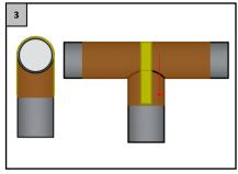
Cut some tecnolato-tape strips that are long enough to cover the tee, as shown in the picture above.
