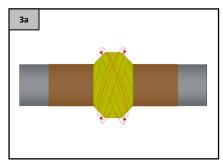
Apply tecnolato-tape, beginning at the center of the flange, and covering the rest by crisscrossing the tapes until there are no uncovered areas left.
