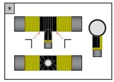
Cut some tecnolato-shield strips and apply them on the angle between pipes, as shown in the picture above.
