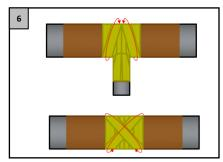
Tighten the tape while placing it in the shape of a cross, as shown in the picture.
