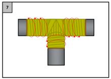
Cover the pipe, placing the tecnolato-tape strips with a 50% overlap, making sure that no air bubbles are generated. If it is necessary, make cuts on the tape to avoid that part of it lifts.
