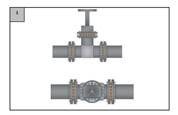
Clean the surface with solvent according to SSPC SP 1. Prepare the Surface with manual cleaning removing every . Prepare the surface manually removing all of the calamine, rust, paint and loose foreign material according to SSPC SP2 or alternatively with mechanical cleaning according to SSPC SP3.
