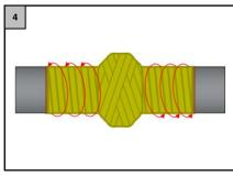
Cover the pipe, placing the tecnolato-tape strips with a 50% overlap, making sure that no air bubbles are generated. If it is necessary, make cuts on the tape to avoid that part of it lifts.
