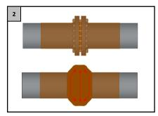
Apply a homogeneous layer of 2-8 mil of tecnolatoprimer over the surface to be covered. Fill the space between the flange faces with tecnolato-mastic. Apply the tecnolato-mastic forming a 45º angle (approximately) between the flange border and the pipe.
