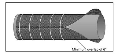
For large diameter pipelines it is recommended that two installers work together with the tape's overlapping, each one located at one side of the pipeline.
