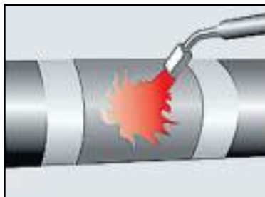
Figure 3: Preheating of the surface
