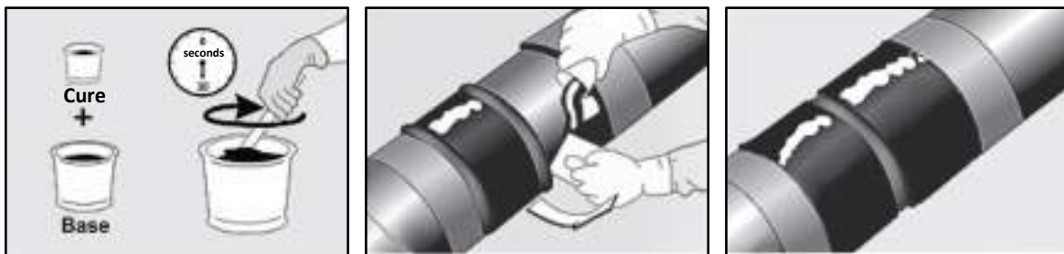
Figures 4, 5 and 6: tecnosleeve-epoxy application
