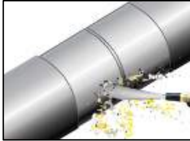
Figure 2: NACE 2/ SSPC-SP10 Near-white metal blast cleaning
