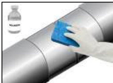
Figure 1: SSPC SP1 Solvent cleaning
