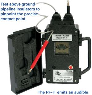
beep. When the operator gets closer to the point of contact the unit starts beeping faster. At the same time, the LCD meter moves from left to right.
