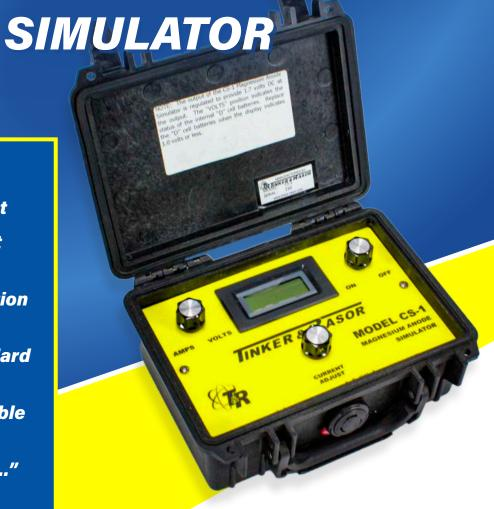
The CS-1 portable Mag. Anode Simulator is an ideal DC current source that will allow the user to see what the addition of a mag anode on their system will do to Pipe to Soil measurements and other CP tests.
