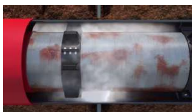
Gel System: Gel crystals are introduced prior to injection through the vent pipes.
