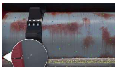
Inhibitors neutralize contaminants on contact and in the vapor space of the annulus. The amount of VCI required depends on the volume of the annulus and any contaminants that may be present.
