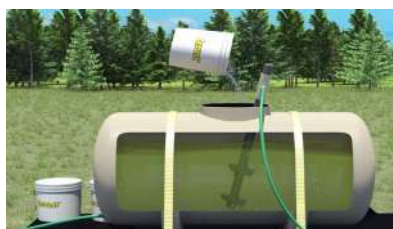
Gel System: Gel crystals are introduced prior to injection through the vent pipes.
